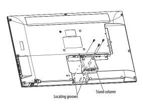
**3** Make sure that the wide portion of the stand base faces the front of your TV, align the base to the stand column, then secure the base to the column with the provided screw.
