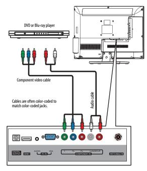
3 Connect an audio cable to the AUDIO L/R jacks next to the COMPONENT IN jacks on your TV and to the L/R AUDIO OUT jacks on the component video device.
