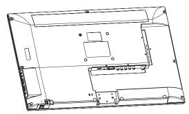
2 Align the locators on the stand column with the locating grooves on the TV back and secure the stand column to your TV with the three provided screws.
