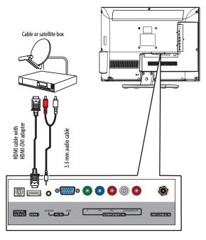
5 Connect a 3.5 mm audio cable (not included) to the PC AUDIO IN jack on your TV and to the AUDIO OUT jack on the cable or satellite box.
