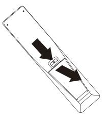
2 Insert two AAA batteries into the battery compartment. Make sure that you match the + and - symbols on the batteries with the + and - symbols in the battery compartment.
